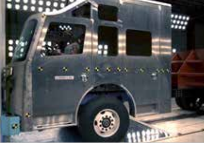
Frontal Impact Test
