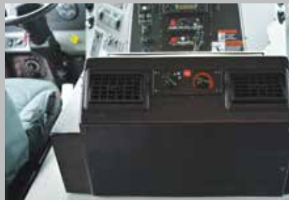
Engine Tunnel HVAC
