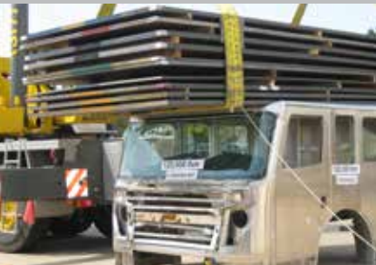
120,000 lb. Crush Test
