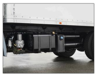
The K270 and K370 has been designed to maximize your payload potential. Starting at only 10,000 pounds, this light weight yet extremely durable chassis features proven North American-supplied components assembled with the meticulous care and craftsmanship that marks Kenworth quality. Constructed of 120,000 PSI-rated steel, the frame provides a 34-inch rail spacing.
