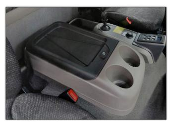
The optional single passenger seat configuration also offers a large locking center console that conveniently consolidates additional storage, cup holders, parking brake, control knob for master display functions, 12 volt power supply and the allnew push button shifting system for Allison automatic transmissions.
