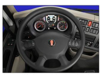
Kenworth's multi-function steering wheel puts the most frequently used controls — cruise control and engine brake — right under the driver's fingertips. The adjustable steering column telescopes in or out and tilts the wheel up or down for a personalized fit.
