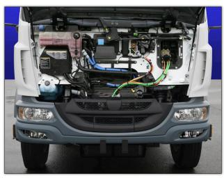
With daily maintenance checks this easy, your K270 and K370 can clock into work right on schedule. Merely open the front access panel and — with feet firmly on the ground — you can check the levels and fill engine oil, coolant and washer fluid.
