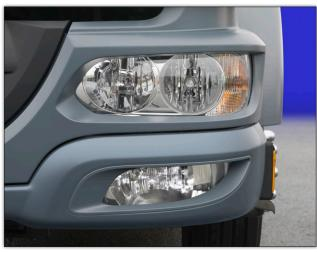
State-of-the-art complex reflector headlamps project a light beam farther and more evenly down the road, increasing the safety of night driving. Replacement bulbs are inexpensive and readily available at your local dealer or auto parts store. Fog lamps come standard for even greater forward visibility.
