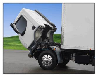
In just seconds — thanks to a hydraulic assist cab tilt of 55 degrees — your mechanic has complete and unfettered access to the engine, transmission, air filter and power steering reservoir.
