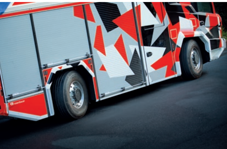
Parallel positioning of the wheels on both axles for maneuvers in confined spaces.
