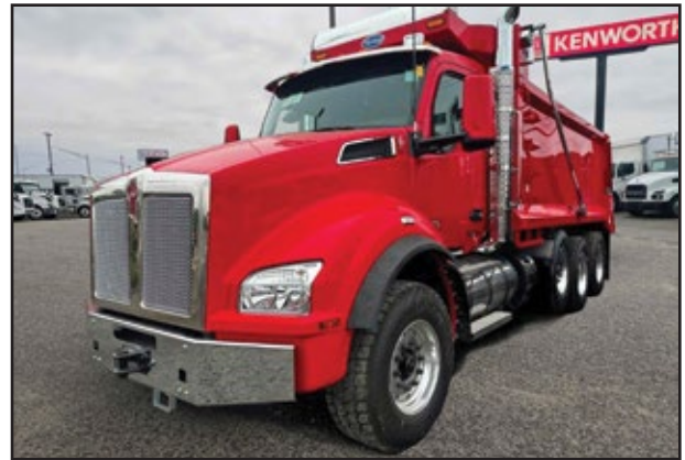
(2) 2025 KENWORTH T880, 565 HP Cummins X15 Engine, EXDP18F118D Transmission, 20,000 Front Axle, 46,000 Rear w/Spring Suspension, Strbl Pshr, 17.6' Heritage Dump. UNIT# RN-3833 Dayton , RN-3830 Dayton
