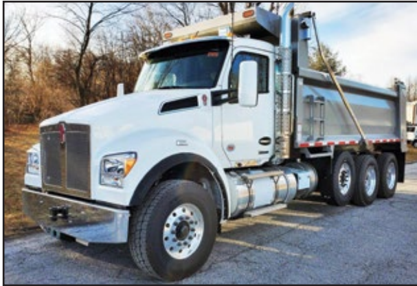
(2) 2025 KENWORTH T880s, 455 HP Paccar MX-13 Engine, PXDP16F118D Automated Transmission, 20,000 Front Axle, 46,000 Rear w/Air Suspension, Strbl Pshr, 18' Brandon Dump. UNIT# DN-4142 Montgomery , DN-4152 Monticello
