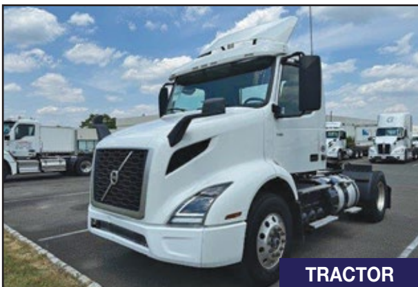
2021 VOLVO VNR42T, 385 HP D11 Volvo Engine, I-Shift Transmission, 12,000 Front Axle, 23,000 Rear w/Air Ride, 156" WB. 68,589 Miles. UNIT# U-277951 Jamaica .....$56,500
