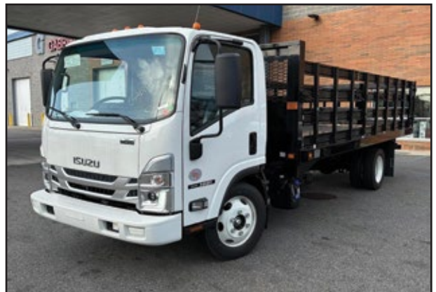
2024 ISUZU NQR, 215 HP Isuzu Diesel Engine, Automatic Transmission, 17,950 GVW, 18' Platform Body. UNIT# NH-0268 Bronx
