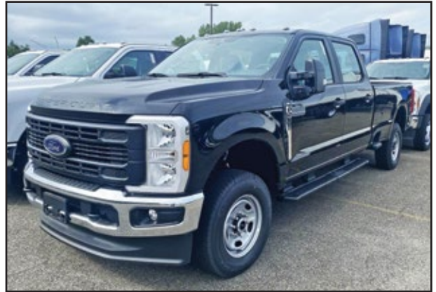
2023 FORD F250 Crew Cab 4x4, 6.8L Gas Engine, Automatic Transmission, 10,000 GVW, 8' Bed. UNIT# BF-4219 Jamaica, BF-4248 Medford
