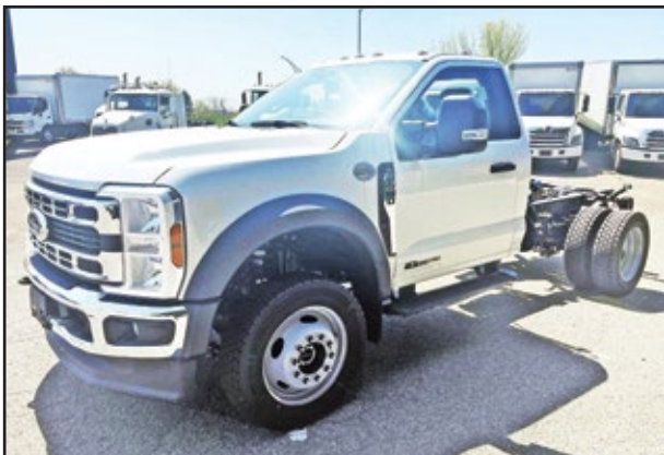
2024 FORD F550 4x4, 6.7L Diesel Engine, Automatic Transmission, 19,500 GVW, 145" WB, 60" CA. UNIT# NF-8669 Medford
