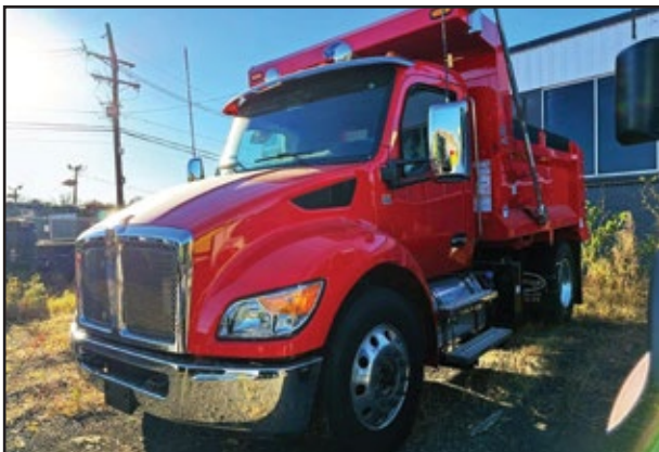
2025 KENWORTH T380, 330 HP PX-9 Engine, 3000 RDS Transmission, 33,000 GVW w/Spring Suspension, 10' Heritage Dump. UNIT# DN-4116 Fairview
