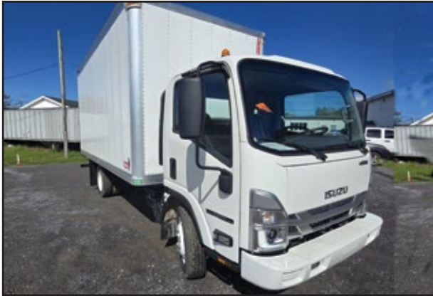
2024 ISUZU NPR-HD, 6.6L 350 HP V8 Gas Engine, Automatic Transmission, 14,500 GVW, 16' 91h x 96w Kidron Body.
