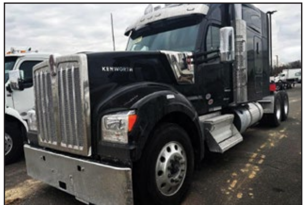
2025 KENWORTH W990, 565 HP Cummins X15 Engine, RTL020918B Transmission, 13,200 Front, 40,000 Rear w/Air Susp, High Roof Sleeper.
