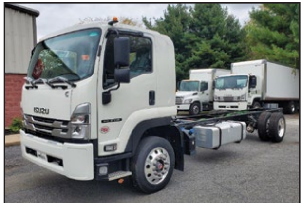
2025 ISUZU FTR LP, 260 HP Cummins B6.7 Engine, Allison Transmission, 25,950 GVW w/Spring Suspension, 224" WB, 199" CA.
