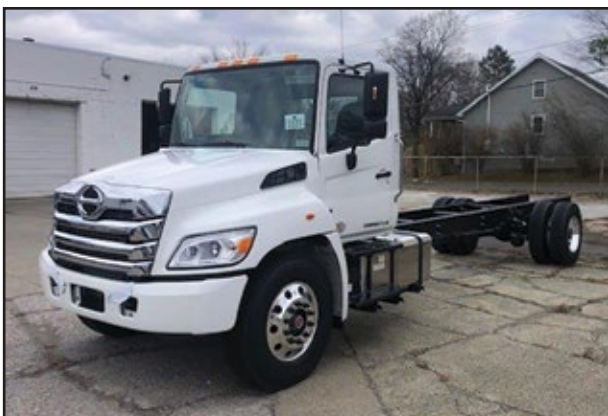
(2) 2025 HINO L6 Ext Cab, 260 HP Cummins, 2500 RDS Transmission, 25,950 GVW w/Air Suspension, 301" WB, 204" CA.
