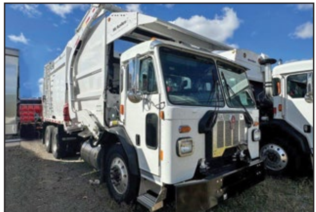
2024 KENWORTH L770, 400 HP Paccar MX-11 Engine, 4500 RDS Transmission, 20,000 Front Axle, 52,000 Rear w/ Spring Suspension, McNeilus 28 Yrd Front End Loader. UNIT# RN-3416 Medford
