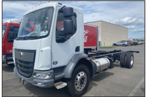
(2) 2024 KENWORTH K370, 260 HP PX-7 Engine, 3000 RDS Transmission, 33,000 GVW, Spring Suspension, 170" WB, 159" CA. UNIT# NK-6575 Dayton, NK-6576 Dayton
