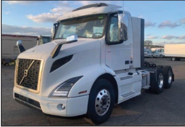
(20) 2025 VOLVO VNR64T300, 435 HP D-13 Volvo Engine, I-Shift Transmission, 12,500 Front Axle, 40,000 Rear w/Air Susp., 176" WB.
