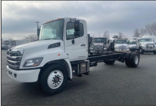
(2) 2025 HINO L6, 260 HP Cummins, 2500 RDS Transmission, 25,950 GVW w/Spring Suspension, 253" WB, 186" CA. UNIT# AH-1027 Albany, NJ-12927 Jamaica
