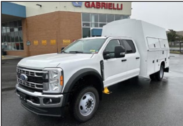
2023 FORD F550 Crew Cab 4x4, 7.3L Gas Engine, Automatic Transmission, 19,500 GVW, 11' Knapheide Utility Body.
