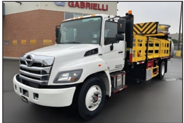
(3) 2025 HINO L6, 260 HP Cummins, 2500 RDS Transmission, 25,950 GVW w/Air Suspension, 18' Scorpion Attenuator Body. UNIT# NH-0502 Hicksville, NH-0507 Medford, NH-0508 Eastern
