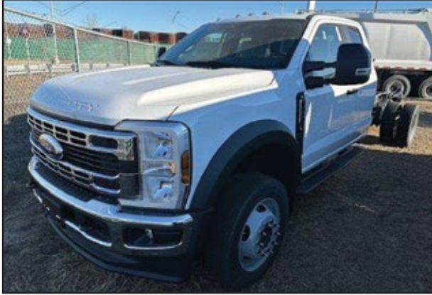
2024 FORD F550 4x4 Super Cab, 7.3L V8 Gas Engine, Automatic Transmission, 19,500 GVW, 192" WB, 84" CA. UNIT# EF-1122 Eastern
