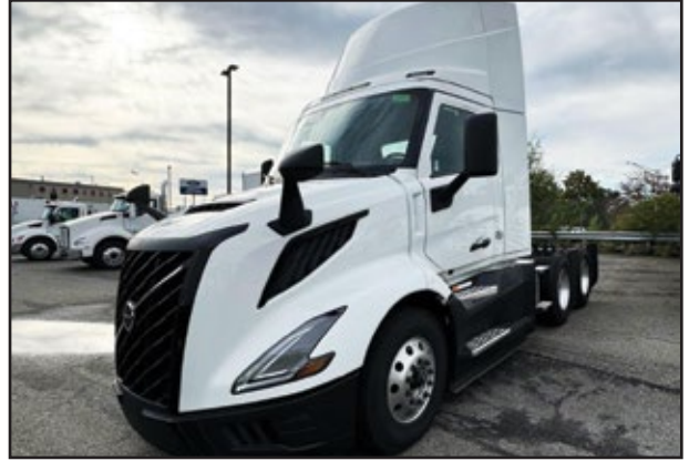
(2) 2025 VOLVO VNL64T300, 455 HP D-13 Volvo Engine, I-Shift Transmission, 12,500 Front Axle, 40,000 Rear w/Air Susp., 171" WB.
