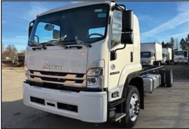
2024 ISUZU FTR LP, 260 HP Cummins B6.7 Engine, Allison Transmission, 25,950 GVW w/Spring Suspension, 224" WB, 199" CA.
