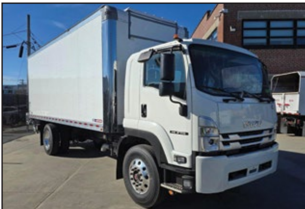
(2) 2024 ISUZU FTR, 260 HP Cummins B6.7 Engine, Allison Transmission, 25,950 GVW w/Air Suspension, 22' Morgan Reefer Body w/Lift Gate.
