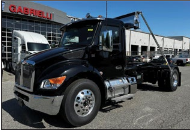
2025 KENWORTH T380, 330 HP PX-9 Engine, 3000 RDS Transmission, 33,000 GVW w/Spring Suspension, Ampliroll AL102S-14 Hooklift. UNIT# DN-4106 Bronx
