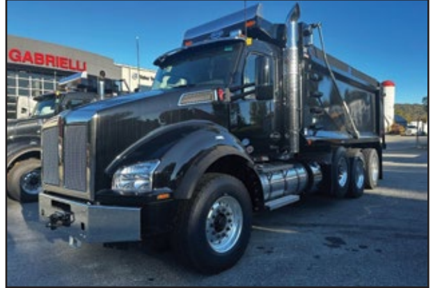
(3) 2025 KENWORTH T880, 565 HP Cummins X15 Engine, EXDP18F118D Transmission, 20,000 Front Axle, 46,000 Rear w/Spring Suspension, Strbl Pshr, 17.6' Heritage Dump. UNIT# RN-3845 Bloomsbury, RN-3841 Bloomsbury, RN-3935 Bloomsbury
