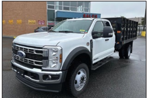
2024 FORD F450 Supercab 4x4, 6.7L Diesel Engine, Automatic Transmission, 16,000 GVW, 12' Knapheide Rack Body.
