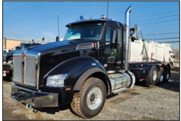
2025 KENWORTH T880, 500 HP Cummins X15 Engine, RTO16908LL 10 Spd, 20,000 Front Axle, 46,000 Rear w/ Spring Suspension, Strbl Pshr, 75k# American Roll Off. UNIT# RN-3681 Ridgefield
