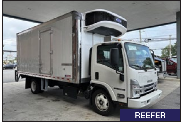
(3) 2023 ISUZU NQR, 215 HP Isuzu Diesel Engine, Automatic Transmission, 17,950 GVW, 18' 91h x 96w Morgan Reefer Body. UNIT# RI-1075, RI-1076, RI-1077 Hicksville
