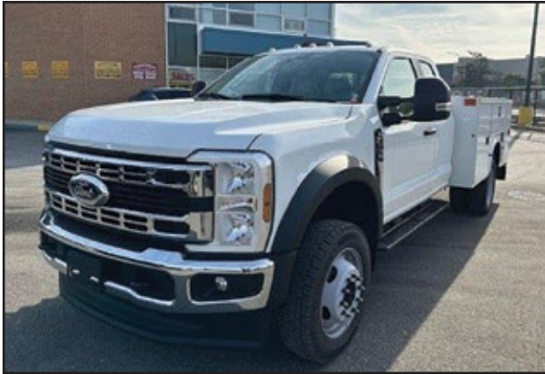
2024 FORD F450 Super Cab 4x4, 7.3L Gas Engine, Automatic Transmission, 16,500 GVW, 9' Knapheide Service Body.
