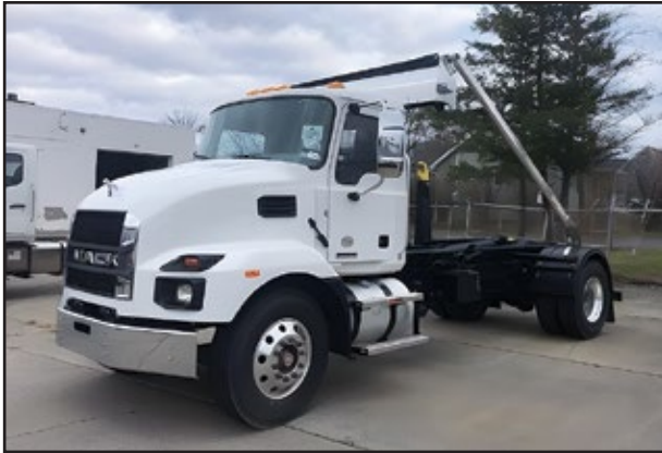
2025 MACK MD742, 300 HP Cummins ISB 6.7-300 D Engine, 3000 RDS Transmission, 25,995 GVW w/Spring Suspension, Ampiroll AL1005-15 Hooklift. UNIT# NJ-12761 Albany
