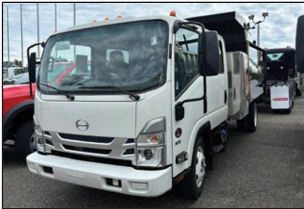
2023 HINO S5-DC Crew Cab, 215 HP Diesel Engine, Automatic Transmission, 19,500 GVW, 12' Down Easter Landscape Dump.
