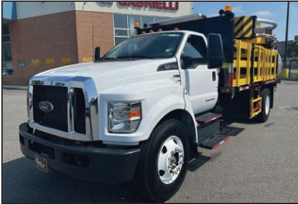
(10) 2025 FORD F650, 7.3L Gas Engine, Automatic Transmission, 25,999 GVW, 15' TMA 3 Scorpion Attenuator Body. UNIT# NF-8643 Hicksville, NF-8645 Milford, NF-8644 Medford, NF-8647 Milford, NF-8649 Milford, NF-8659 Jamaica, NF-8660 Medford, NF-8663 Jamaica, NF-8664 Eastern
