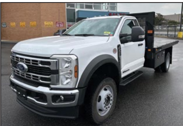
2024 FORD F450 4x4, 6.7L Diesel Engine, Automatic Transmission, 16,500 GVW, 12' Knapheide Platform Body.
