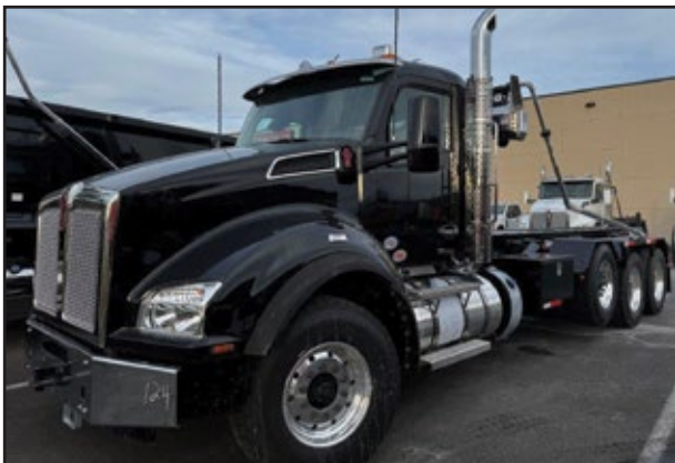
2025 KENWORTH T880, 500 HP Cummins X15 Engine, RTO16908LL 10 Spd, 20,000 Front Axle, 52,000 Rear w/ Air Suspension, Strbl Pshr, 75k# American Roll Off. UNIT# RN-3804 Dayton
