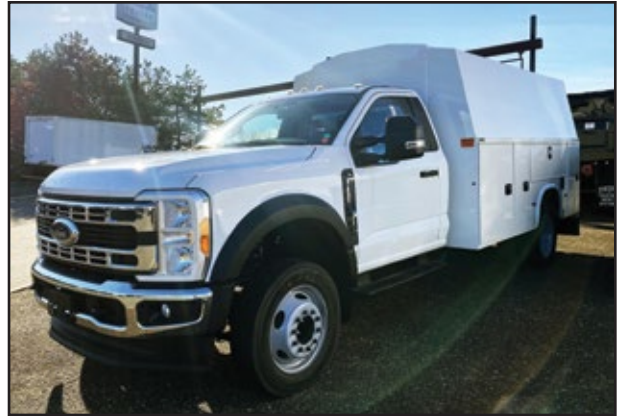
2023 FORD F550, 7.3L Gas Engine, Automatic Transmission, 19,500 GVW, 11' Knapheide KUV Utility Body.
