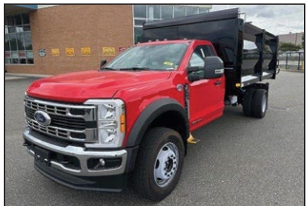
2023 FORD F600 4x4, 6.7L Diesel Engine, Automatic Transmission, 22,000 GVW, 14' Rugby Landscape Dump. UNIT# EF-1076 Milford
