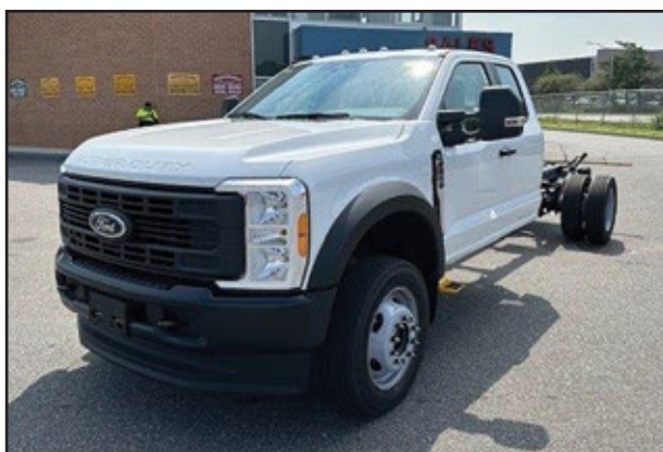
2024 FORD F550 4x4 Super Cab, 7.3L V8 Gas Engine, Automatic Transmission, 18,000 GVW, 192" WB, 84" CA.
