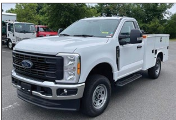
2023 FORD F250 4x4, 6.8L Gas Engine, Automatic Transmission, 10,000 GVW, 9' Knapheide Service Body. UNIT# EF-1059 Milford
