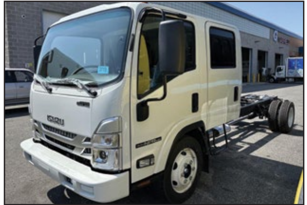
2024 ISUZU NPR HD Crew Cab, 6.6L 350 HP V8 Gas Engine, Automatic Transmission, 14,500 GVW, 176" WB, 153" CA.
