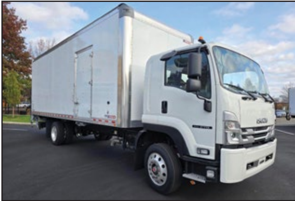
2025 ISUZU FTR LP, 260 HP Cummins B6.7 Engine, Allison Transmission, 25,950 GVW w/Air Suspension, 26' 103h x 102w Morgan Body w/Lift Gate.
