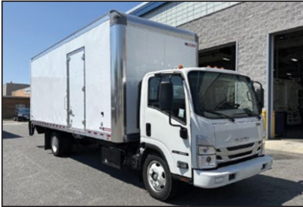
2024 ISUZU NRR, 215 HP Diesel Engine, Automatic Transmission, 19,500 GVW, 22' 97h x 91w Morgan Body w/Lift Gate.
