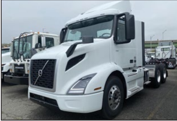
(2) 2025 VOLVO VNR64T300, 425 HP D-13 Volvo Engine, I-Shift Transmission, 12,000 Front Axle, 40,000 Rear w/Air Susp., 183" WB.
