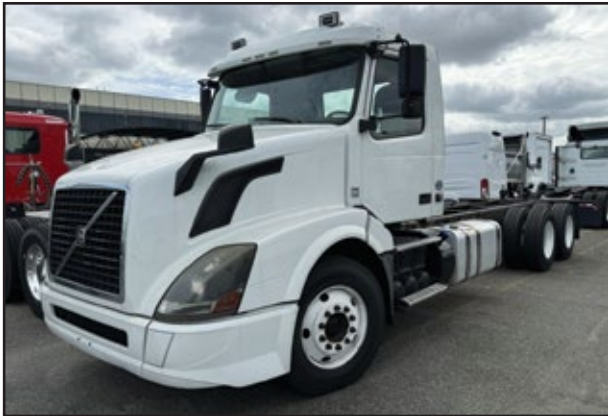
2017 VOLVO VNL, 405 HP D11 Engine, 10 Spd Manual Transmission, 16,000 Front Axle, 40,000 Rear Axle w/Air Suspension, 215 WB, 148" CA. UNIT# UD-1664 .....$60,500
