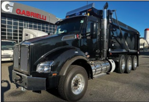
(2) 2025 KENWORTH T880, 565 HP Cummins X15 Engine, 4500 RDS Transmission, 20,000 Front Axle, 46,000 Rear w/Spring Suspension, Strbl Pshr, 17.6' Heritage Dump. UNIT# RN-3868 Bloomsbury, DN-6003 Eastern
