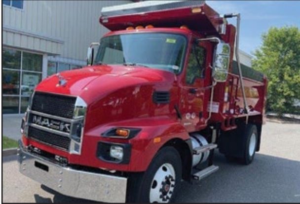
2025 MACK MD742, 300 HP Cummins ISB 6.7-300 D Engine, 2500 RDS Transmission, 33,000 GVW w/Spring Suspension, 11.5' Beau Roc Dump. UNIT# HM-1491 Milford
