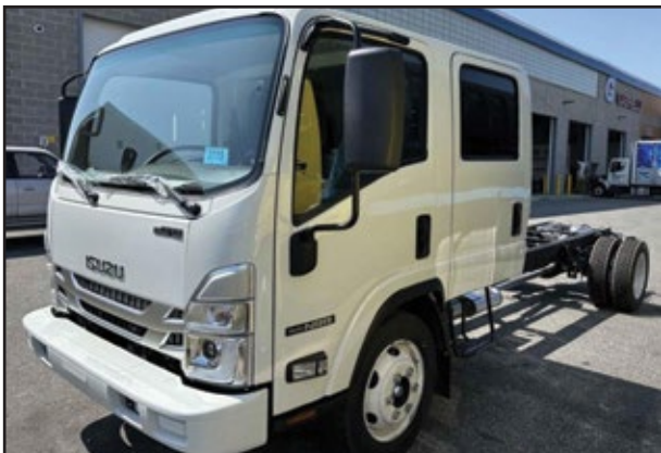
2024 ISUZU NRR Crew Cab, 6.6L 350 HP Gas Engine, Automatic Transmission, 19,500 GVW, 176" WB, 153" CA.
