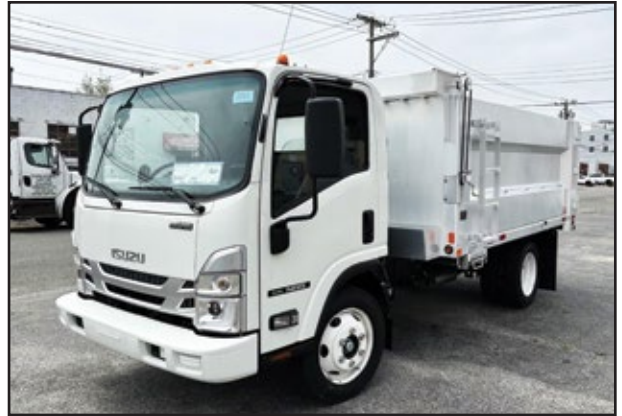
2024 ISUZU NRR, 6.6L 350 HP V8 Gas Engine, Automatic Transmission, 19,500 GVW, 12' Voth Aluminum Dump Body.
