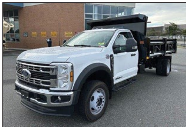
2024 FORD F550 4x4, 6.7L Diesel Engine, Automatic Transmission, 19,500 GVW, 14' Rugby Dump. UNIT# EF-1125 Eastern
