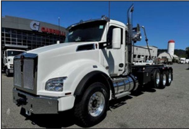
2025 KENWORTH T880, 500 HP Cummins X15 Engine, RTO16908LL 10 Spd, 20,000 Front Axle, 46,000 Rear w/ Spring Suspension, Strbl Pshr, 75k# American Roll Off. UNIT# RN-3806 Bloomsbury
