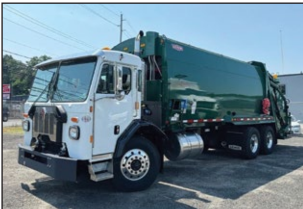
2024 KENWORTH L770, 400 HP Paccar MX-11 Engine, 4500 RDS Transmission, 20,000 Front Axle, 52,000 Rear w/ Spring Suspension, 32 Yrd Leach Rear Loader. UNIT# RN-3388 Fairview
