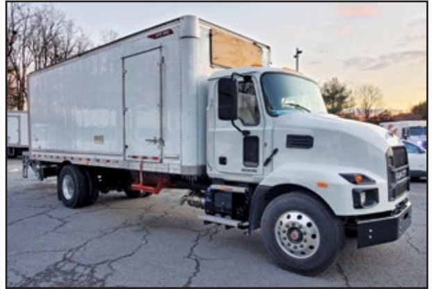
(8) 2024 MACK MD642, 260 HP Cummins ISB 6.7-260 D Engine, 2500 RDS Transmission, 25,995 GVW w/Air Suspension, 22' 97h x 96w Alpine Reefer Body w/Lift Gate. UNIT# NJ-12658 Montgomery, NJ-12670 Montgomery, NJ-12689 Jamaica, NJ-12714 Jamaica, NJ-12764 Jamaica, NJ-12837 Fairview
