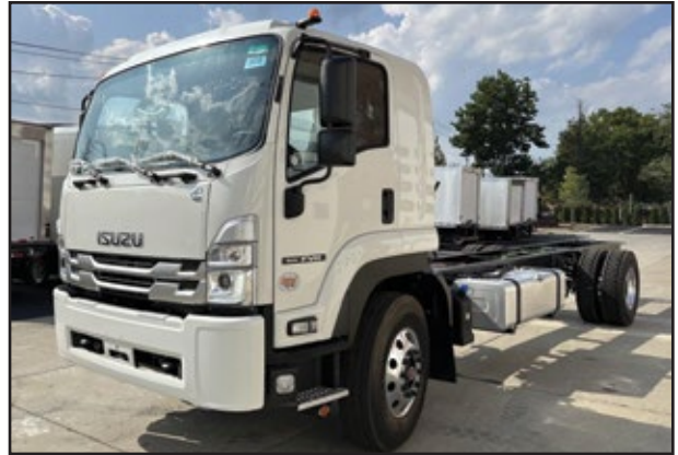
2025 ISUZU FVR, 260 HP Cummins B6.7 Engine, Allison Transmission, 25,950 GVW w/Spring Suspension, 224" WB, 199" CA.
