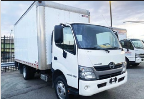
(3) 2016 HINO 195, 210 HP Engine, Automatic Transmission, 19,500 GVW, 16' 91h x96w Morgan Body w/Lift Gate.
