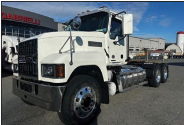
(3) 2025 MACK PI64T, 445 HP Mack MP8 Engine, M-Drive Transmission, 14,600 Front Axle, 46,000 Rear w/Air Suspension, 213" WB. UNIT# NJ-13028 Bloomsbury, NJ-13031 Milford, NJ-13061 Rockaway
