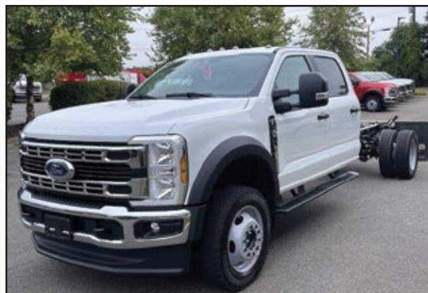
2024 FORD F550 Crew Cab, 7.3L Gas Engine, Automatic Transmission, 19,500 GVW, 203" WB, 84" CA. UNIT# EF-1119 Milford
